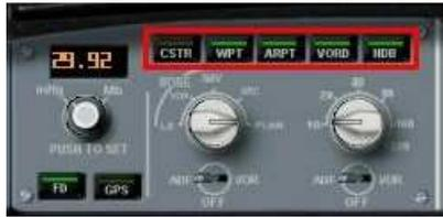
L'EFIS (Electronic Flight Instrument System) Control...
